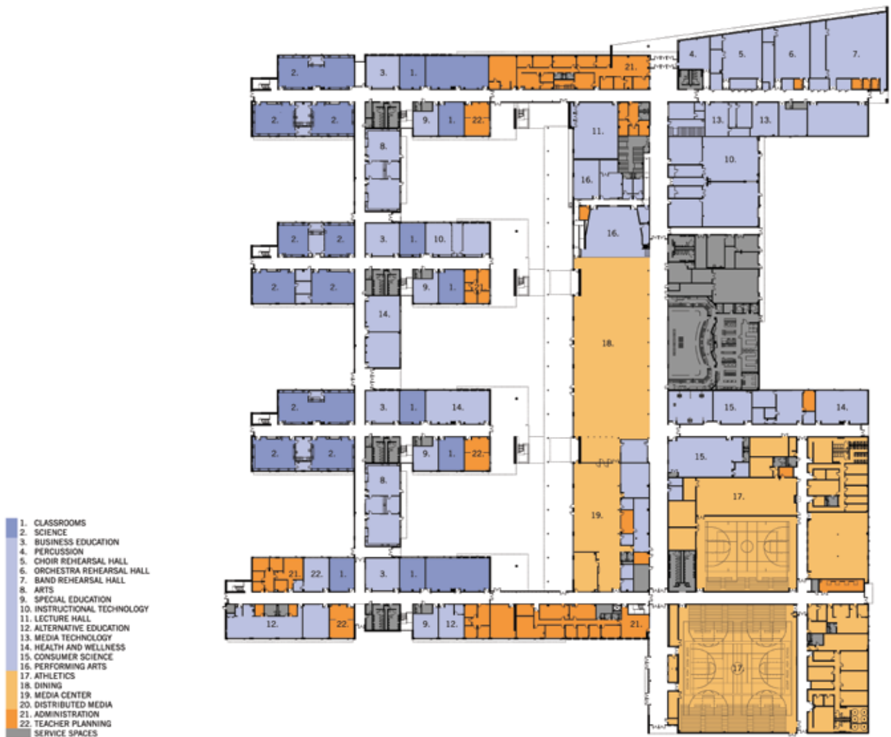
This floor plan demonstrates the concept of breaking up a large high school into small learning community groups that encourage more interaction and make the school less overwhelming. Diagram: Perkins+Will
